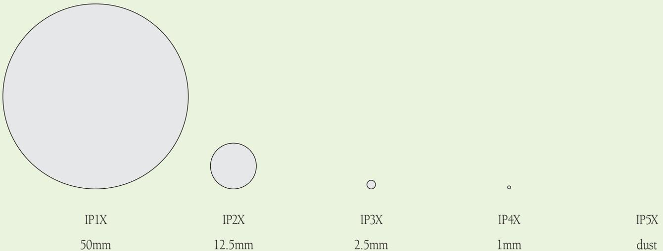
To get some notion of how big the “foreign objects” being described in each of these ratings really are, the diagram above shows actual particle sizes. This shows that an AED like the Philips HeartStart OnSite, because it has a rating of IP21, is in danger of being compromised by a small pebble about 1/2 inch in diameter.
